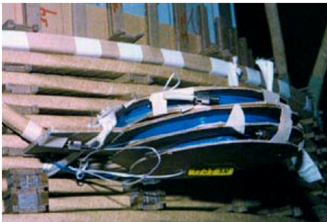
Fig. 6 Temporary spooling of fiber optic sensor
